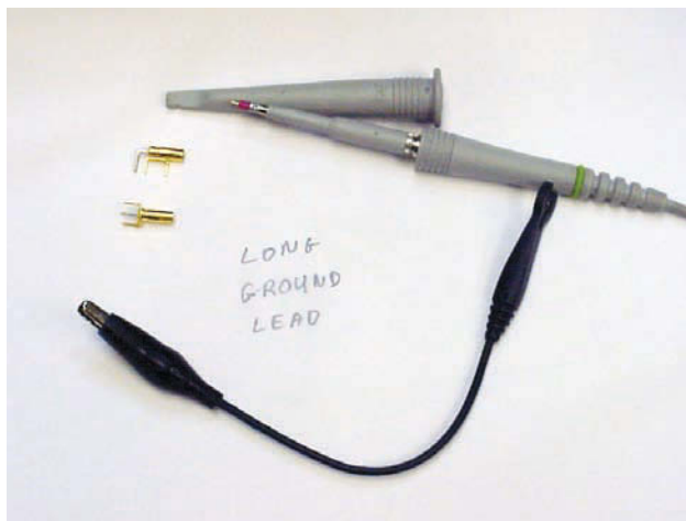
Figure 1 A standard oscilloscope probe has a ground lead that can pick up noise.
